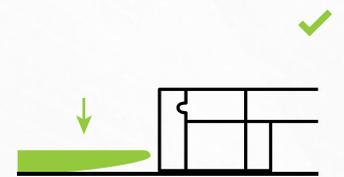
Insert the forks completely and lift to move. Do not drag or push the pallet.
